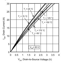
Figure 2 • Drain Current vs. Drain-to-Source Voltage
