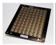
The W9502RC adapter is now available in panel format, where the circuit is step and repeated to enable processing in an automatic production environment.
