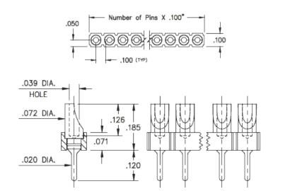
**Description:** Interconnect Header Solder Tail Pin Header SolderCup Head Single Row Through Hole Plating Code: 10 Shell Plating: 10  $\mu$ " Gold over 100  $\mu$ " Nickel
