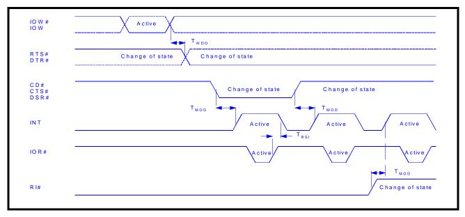
FIGURE 16. 16 MODE (INTEL) DATA BUS READ TIMING FOR CHANNELS A-D
