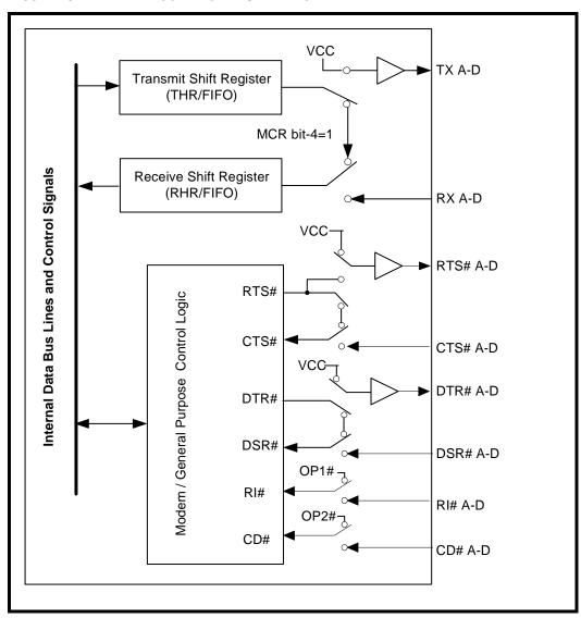
FIGURE 13. INTERNAL LOOP BACK IN CHANNELS A-D
