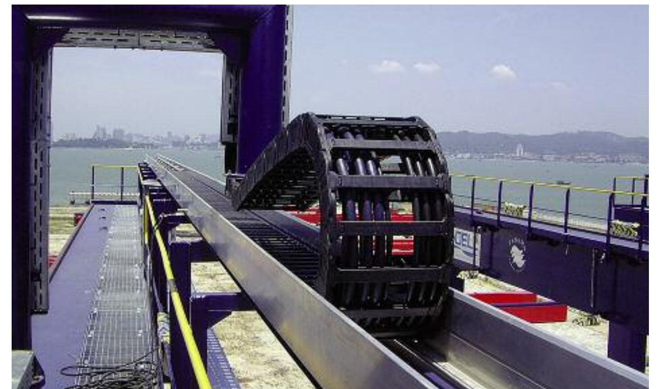
chainflex® CF9 for outdoor crane systems. e-chain®: Series E4/00
