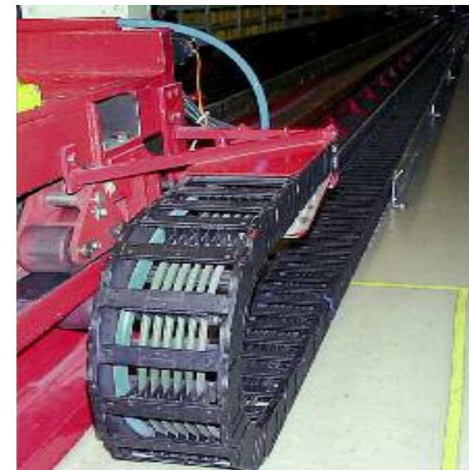
chainflex® CF5/CF6 for shelf control units: long travel in the longitudinal axis. e-chain®: Serie E4/00 with igus® guide trough out of steel
