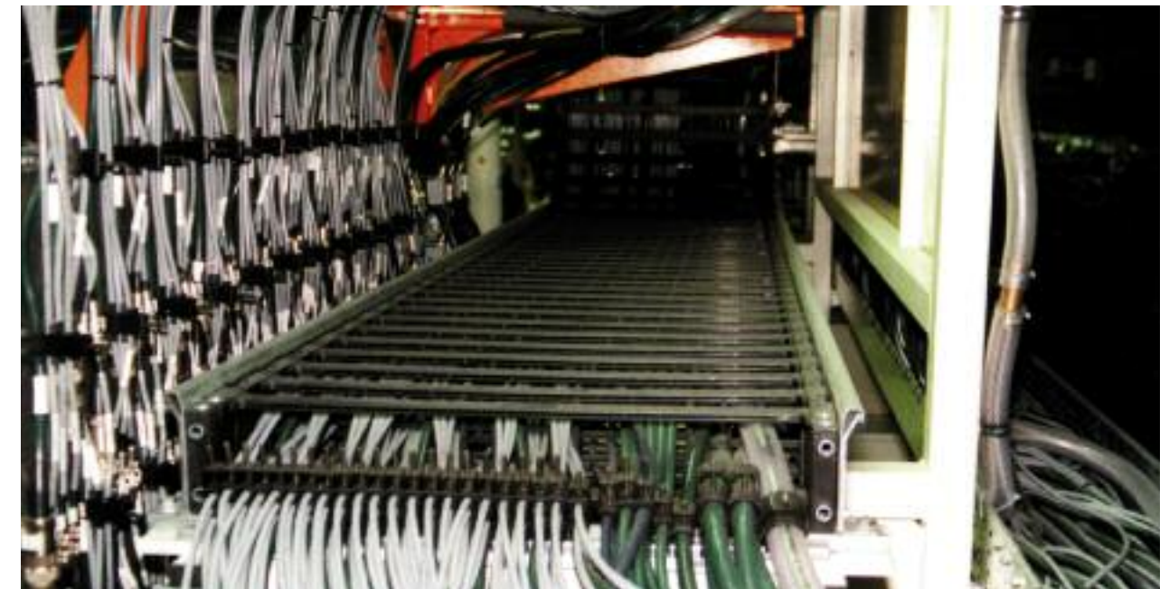
chainflex® CF5 and CF6 control cable (green) as well as CF211 measuring system cable (grey) in a screwing station of a motor factory. e-chain®: System E4/00 with chainfix Clip Strain Relief Devices
