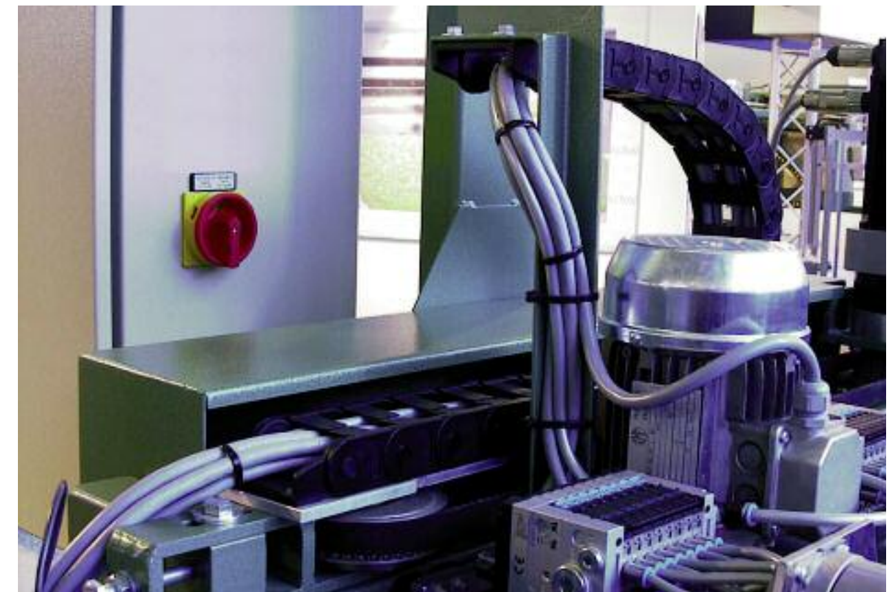
chainflex® CF140.UL for automatic feeder units. e-chain®: easychain®
