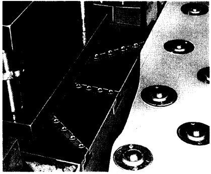
Mounting system of mechanical segment with securing device.
