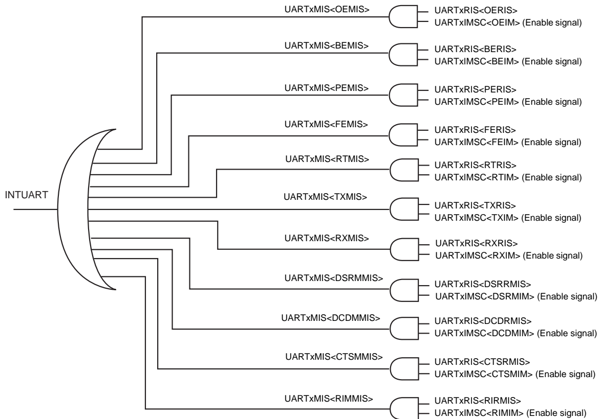
Figure 13-2 UART interrupt block
