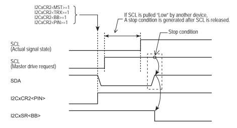
Figure 14-21 Generating the Stop Condition
