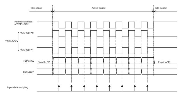
Figure 15-13 Idle period in SIO mode and the transmit pin status
