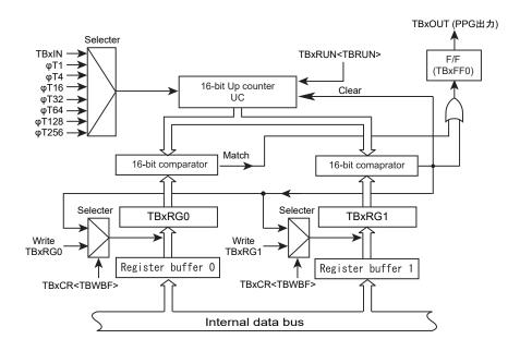
Figure 10-4 Block diagram of 16-bit PPG mode
