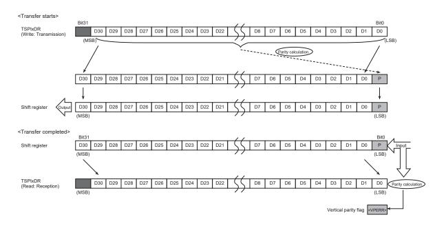
Figure 15-7 MSB first (31-bit data with a parity)
