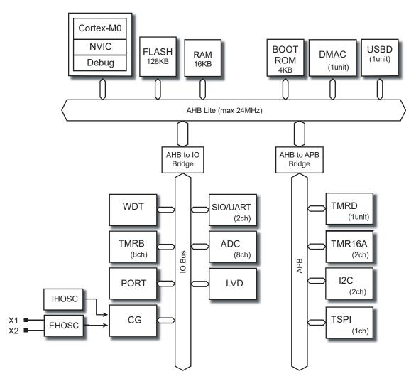
Figure 1-1 Block Diagram
