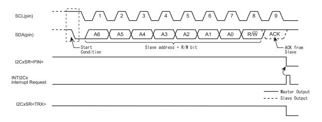
Figure 14-17 Generating the Start Condition and a Slave Address
