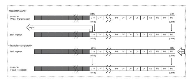
Figure 15-4 MSB first (16-bit data without a parity bit)
