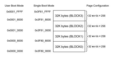
Figure 20-1 Block configuration
