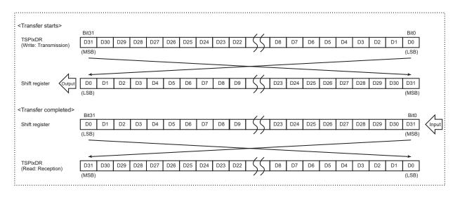
Figure 15-5 LSB first (32-bit data without a parity bit)
