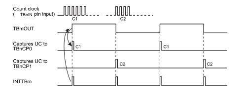
Figure 10-6 Frequency measurement
