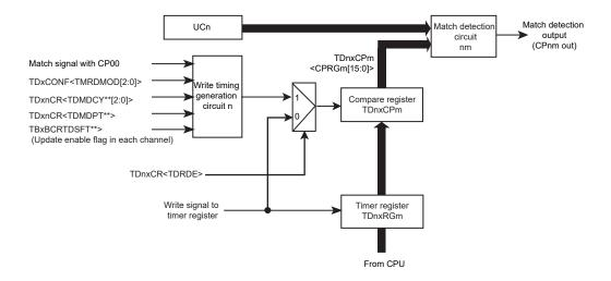
Figure 12-5 Configuration of comparator (CP05)
