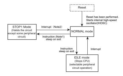
Figure 6-2 Mode Transition Diagram
