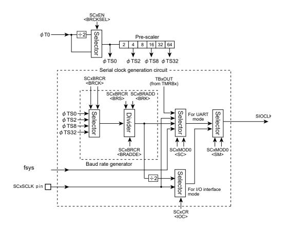
Figure 13-2 Serial clock generation circuit block diagram
