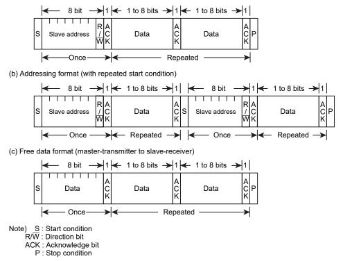
Figure 14-3 I2C Bus Mode Data Formats
