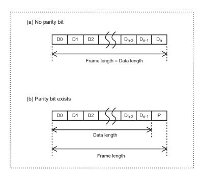
Figure 15-2 Data format schematic
