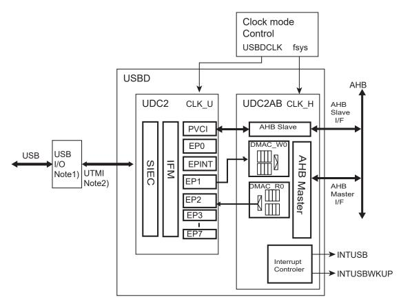
Note1) TMPM066/067/068FW has USB I/O which can be used for Full Speed mode not Low Speed mode. The word "PHY" in this section should be read as USB I/O. Note2) USB2.0 Transceiver Macrocell Interface
