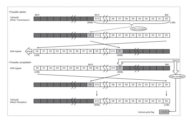
Figure 15-10 LSB first (15 bits data with parity)
