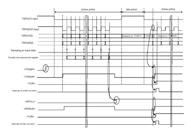
Figure 15-17 Overrun error and under run error
