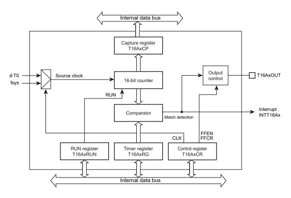
Figure 11-1 Block diagram of TMR16A
