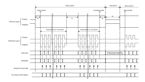
Figure 15-11 Transfer format and timing adjustment
