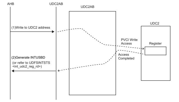
Access flow diagram for UDC2 register is shown below.
