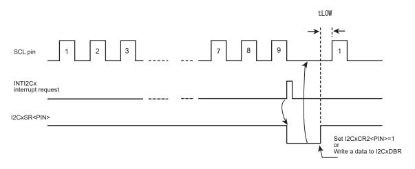
Figure 14-10 I2CxSR<PIN> and SCL
