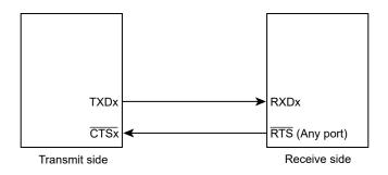
Figure 13-11 Handshake Function
