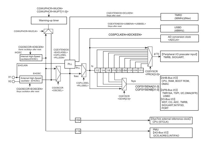
Figure 6-1 Clock Block Diagram
