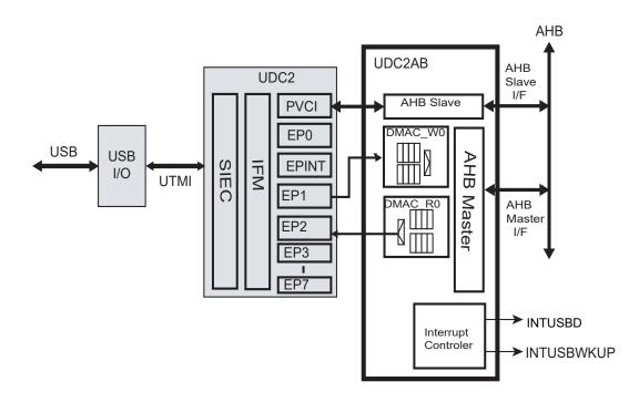
Figure 16-2 UDC2AB Block Diagram
