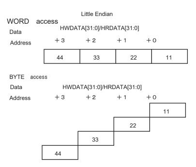
Figure 16-3 Image of Endian conversion in AHB Master function
