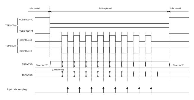
Figure 15-12 Idle period in SPI mode and the transmit pin status
