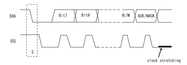
Figure 14-24 Clock stretch Function
