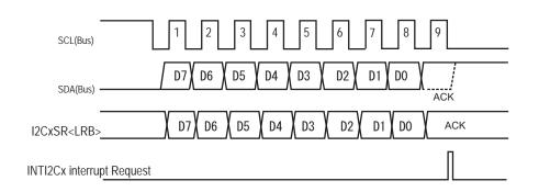
Figure 14-15 Last Received Bit Monitor
