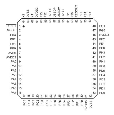
Figure 1-2 Pin Layout (LQFP64 TOP VIEW)
