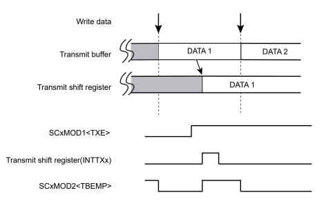
Figure 13-8 Operation of Transmit Buffer (Double-buffer is enabled)
