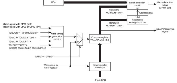
Figure 12-3 Configuration of comparators (CP02, CP04, CP12, CP14)
