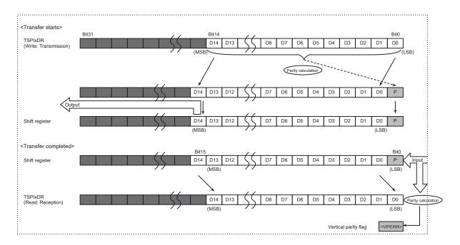
Figure 15-8 MSB first (15 bits data with parity)
