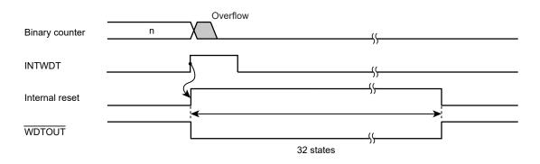
Figure 19-3 Internal reset generation
