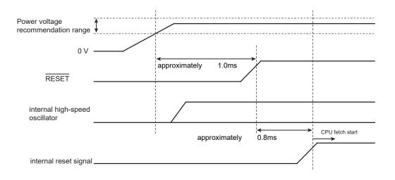
Figure 5-1 Cold reset Operation Sequence
