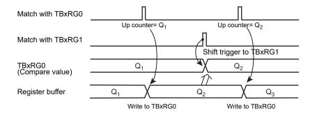
Figure 10-3 Register buffer operation
