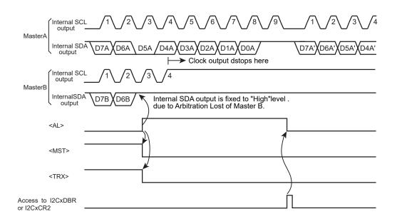
Figure 14-12 Example of Master B Lost Arbitration (D7A = D7B, D6A = D6B)
