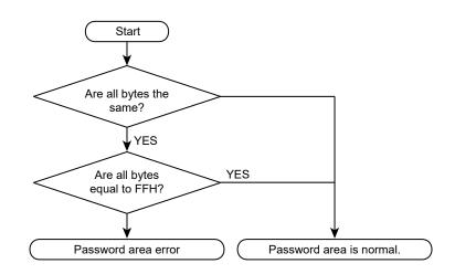
Figure 20-9 Password area check flowchart
