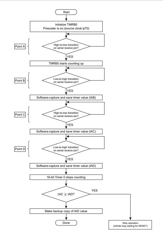
Figure 20-7 Serial operation mode receive flowchart
