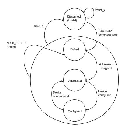
Figure 16-21 Device state diagram
