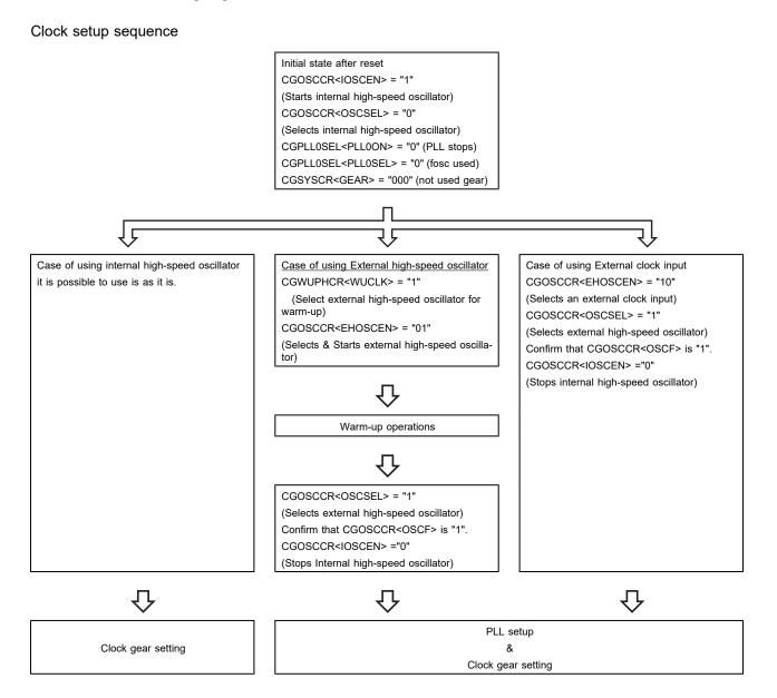
Note: When an internal high-speed oscillator is used as fsys, the usage of PLL function is prohibited.
