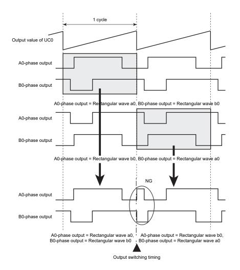
Figure 12-21 Waves before/after phase advance/delay (output SW) (A trailing edge of rectangular wave PPG10 is over the UC0 cycle.)
