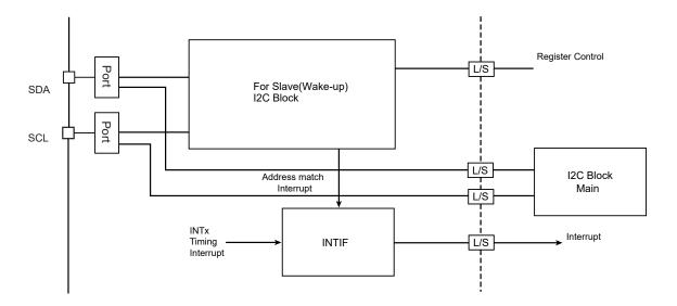
Figure 14-23 Wake-up Function Block
