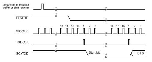
Figure 13-12 SCxCTS Signal timing
