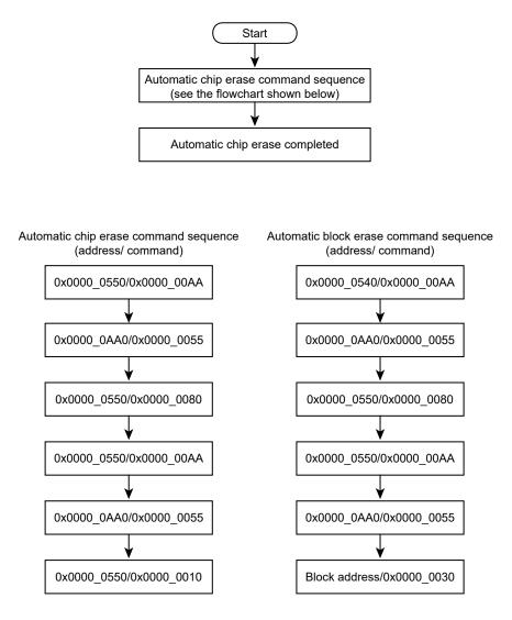
Figure 20-5 Flowchart of automatic erase
