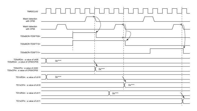
Figure 12-18 A timing to set update enable register is delayed than a match with CP05
