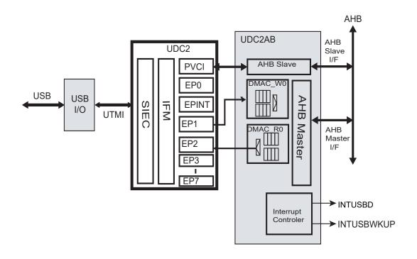
Figure 16-5 Block diagram of UDC2
