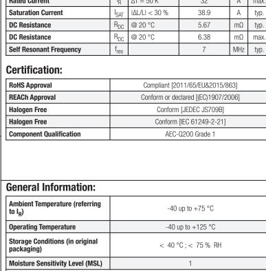
Test conditions of Electrical Properties: +20 °C, 33 % RH if not specified differently
