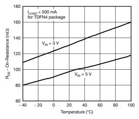
Fig. 12 - R<sub>DS(on)</sub> vs. Temperature
