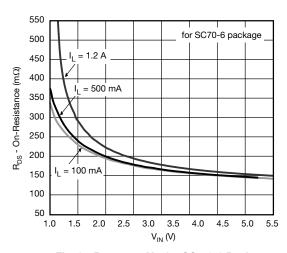
Fig. 8 - R<sub>DS(on)</sub> vs. V<sub>IN</sub> for SC-70-6 Package
