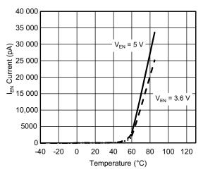
Fig. 15 - I<sub>EN</sub> Current vs. Temperature
