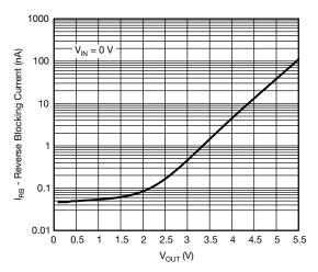
Fig. 10 - Reverse Blocking Current vs. V<sub>OUT</sub>
