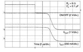
Fig. 16 - Switching (V<sub>IN</sub> = 3 V)
