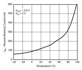
Fig. 13 - Reverse Blocking Current vs. Temperature
