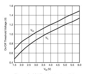
Fig. 14 - On / Off Threshold vs. Input Voltage
