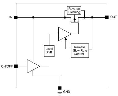
Fig. 20 - Functional Block Diagram
