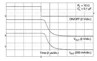
Fig. 17 - Switching (V<sub>IN</sub> = 5 V)
