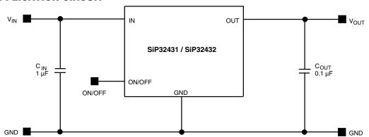
Fig. 1 - SiP32431 / SiP32432 Typical Application Circuit
