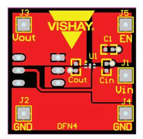
Fig. 21 - Top, TDFN4 1.2 mm x 1.6 mm PCB Layout
