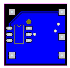
Fig. 22 - Bottom, TDFN4 1.2 mm x 1.6 mm PCB Layout
