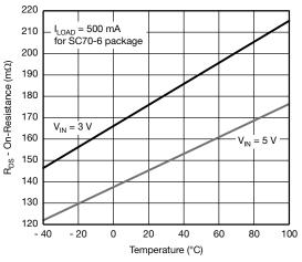
Fig. 11 - R<sub>DS(on)</sub> vs. Temperature
