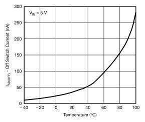
Fig. 7 - Off Switch Current vs. Temperature
