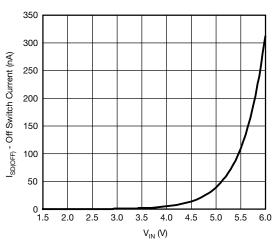
Fig. 5 - Off Switch Current vs. Input Voltage
