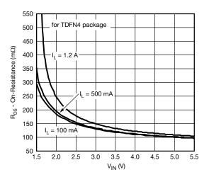
Fig. 9 - R<sub>DS(on)</sub> vs. Input Voltage
