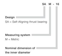
The example shows a spherical thrust bearing with metric dimensions and an inner diameter of 16 mm.
