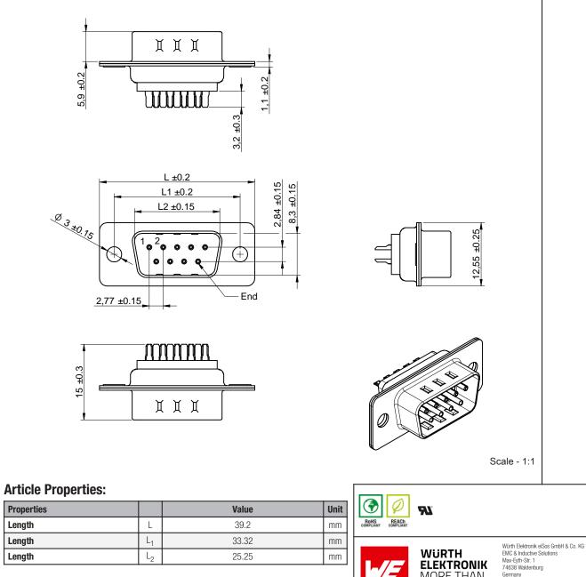
REVISION DATE (YYYY-MM-DD) GENERAL TOLERANCE PROJECTION METHOD (Đ 001.001 2021-07-01 DIN ISO 2768-1m **WR-DSUB Male Solder Bucket** ORDER CODE 61801524823 STATUS BUSINESS UNIT PAGE 1/6 eiCan Valid
