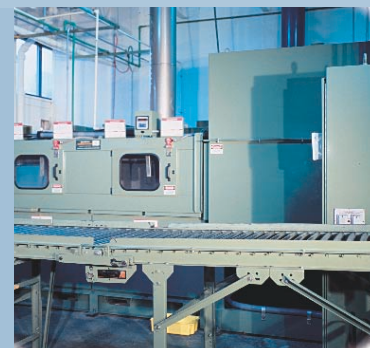
This environment-friendly, aqueous degreasing unit for removing stamping oils cleans with a mild alkaline solution—eliminating the need for chlorinated solvents.
