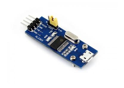
USB TO UART solution with USB micro connector
