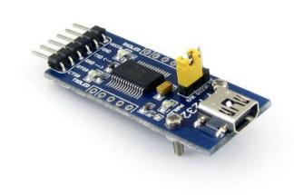
USB TO UART solution with USB mini connector
