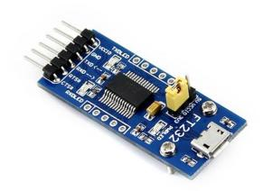
USB TO UART solution with USB micro connector
