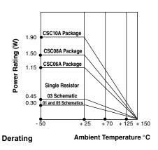
"A" PROFILE +70 °C PACKAGE RATINGS CSC12A 1.5 W 1.37 W CSC11A CSC10A 1.25 W CSC09A 1.12 W CSC08A 1.00 W CSC07A 0.87 W CSC06A 0.75 W CSC05A 0.62 W CSC04A 0.40 W
