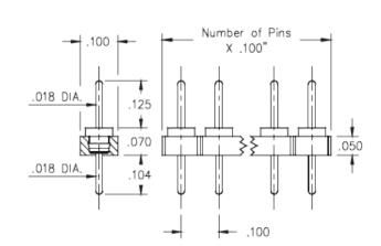
**Description:** Interconnect Header Low Profile Solder Tail Header .018" (0,46mm) Pin Head Single Row Through Hole Plating Code: 40 Shell Plating: 200 µ" Tin (matte finish) over 100 µ" Nickel
