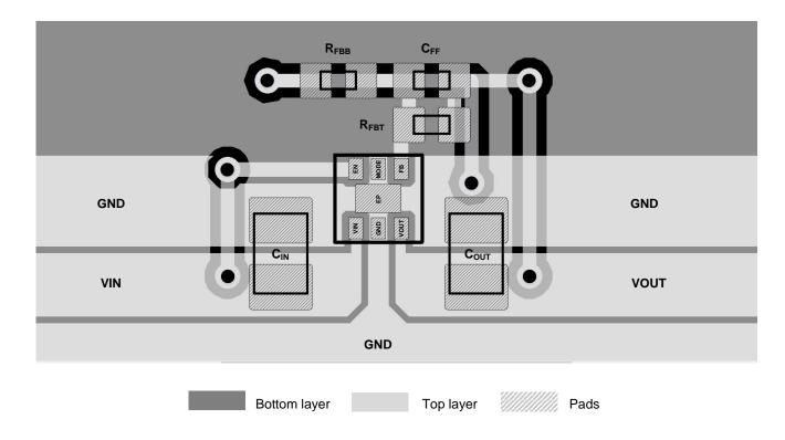
The picture above shows a possible layout for the 171010550 Magl<sup>3</sup>C MicroModule. Nevertheless, some recommendations should be followed when designing the layout:
