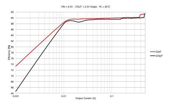
While the recommended  $C_{FF}$  value of 22pF will work for most applications, the user can adjust the performance of the module based on their application by trading between light load efficiency and transient response. This customization tailors the behavior of the module to the application's needs.
