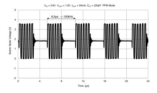
Increasing C<sub>FF</sub> will cause the module to burst more often (shown in the two images above) resulting in a decrease in light load efficiency as depicted in the diagram below. In addition, increasing the C<sub>FF</sub> value will result in an increase in the current threshold required to exit PFM mode, also shown below as a difference of almost 100mA.
