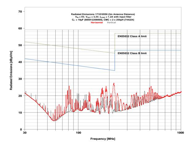
The diagram above refers only to forced PWM mode. Nevertheless similar results would be obtained in PFM/PWM mode because at this load current (1.2A) there is no difference between the two modes.
