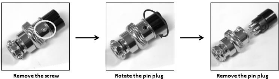
Figure 4 - Remote Control Connector
