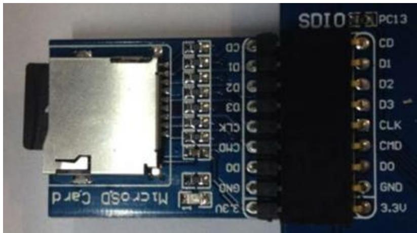
Connect the Micro SD Storage Board to the board via SDIO interface.
