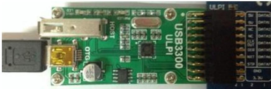
Insert the USB3300 to the ULPI socket
