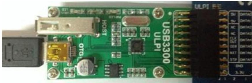
Insert the USB3300 to the ULPI socket
