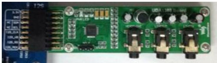
Connect the UDA1380 Board to the board via I2S interface.
