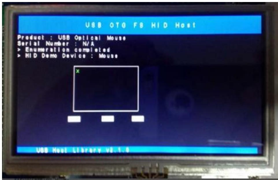
Connect a USB mouse to the on board USB interface through an USB OTG cable
