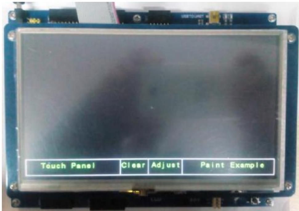
Connect the 7inch Resistive Touch LCD to the board via the LCD interface 1 using 40PIN FFC wire.
