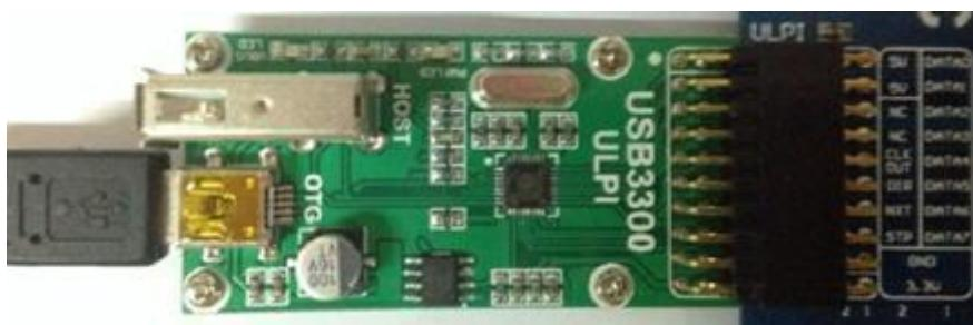
Insert the USB3300 to the ULPI socket
