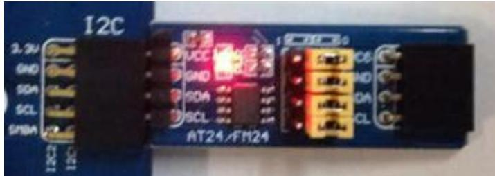
Connect the AT24/FM24 Board to the board via I2C connector (I2C1 or I2C2, depending on the software configuration).
