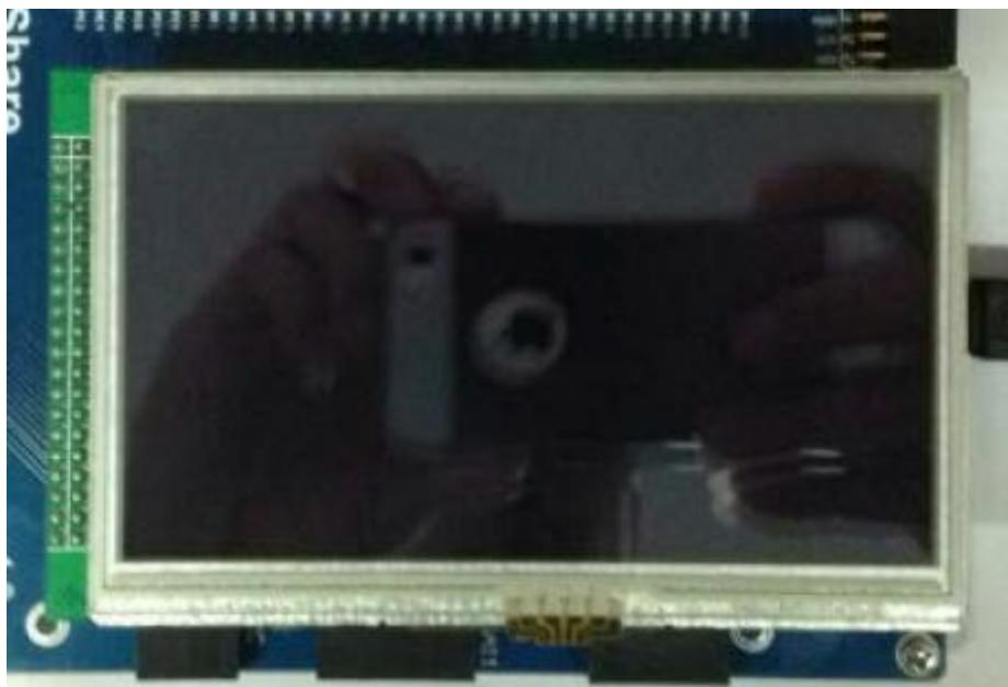
Connect the 4.3inch 480x272 Touch LCD (B) to the board via LCDinterface.
