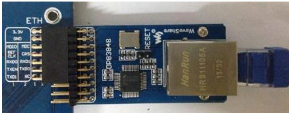
The Ethernet wire connects to the ETH interface and the PC.
