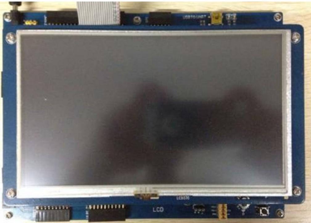
Connect the 7inch Capacitive Touch LCD to the LCD interface 1 using 40PIN FFC wire, and to the Capacitive touch panel interface via 4PIN FFC.
