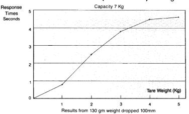
As you can see tare weight increases settling time and should be kept to a minimum.
