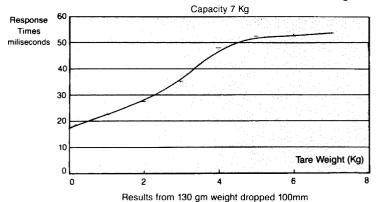
With the 240 Damped Load Cell you can see that the settling time is drastically reduced from more than 1 second to less than 100 m/seconds. (See Fig. 2 and 3.)
