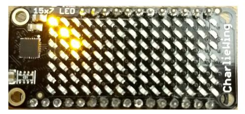
Notice how the first call switches to make frame 1 the active frame but doesn't display it because show is set to false. Then the frame pixel data is changed with fill and pixel commands, and finally the frame is shown by calling frame again but letting the default show = True be used so the frame is displayed.
