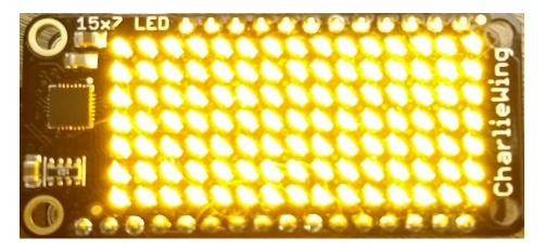
You might notice some buzzing or ringing sounds from the display when all pixels are lit, this is normal as the Charlieplex driver quickly switches LEDs on and off.
