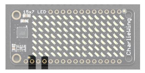
The LED matrix uses only the **3V** (second from left) and **GND** (fourth from left) pins for power and logic. Current draw depends on how many LEDs are lit but you can approximate it as about 40mA for most uses.
