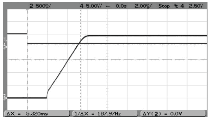
Step Load Transient Response (Vin=5V, Vout=2.5V, Load=0, Iout=3A to 1.5A) Trace 2=Vout, 100 mV/div. Trace 4=Iout, 2.5A/div.
