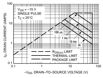
Figure 11. Maximum Rated Forward Biased Safe Operating Area
