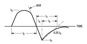
Figure 12. Diode Reverse Recovery Waveform
