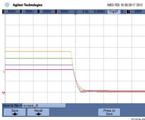
Figure 8. Tracking Supplies Down with DC1978A
