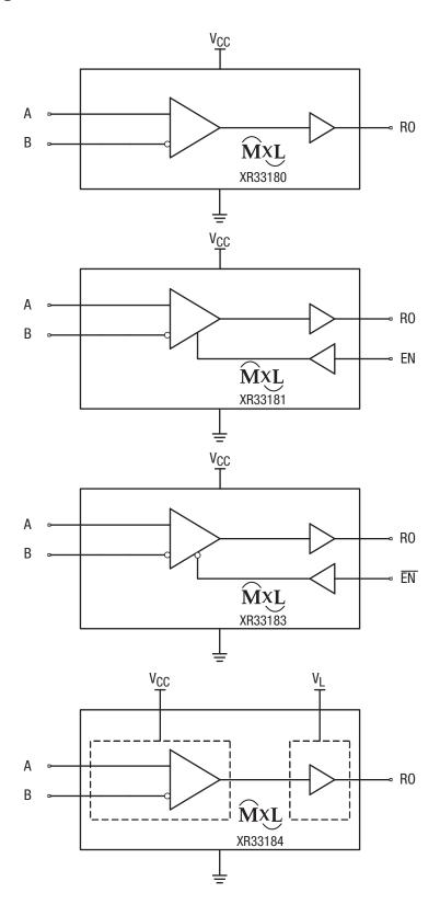
Figure 2. Functional Block Diagrams
