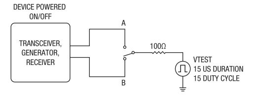
Figure 3. Transient Overvoltage Test Circuit
