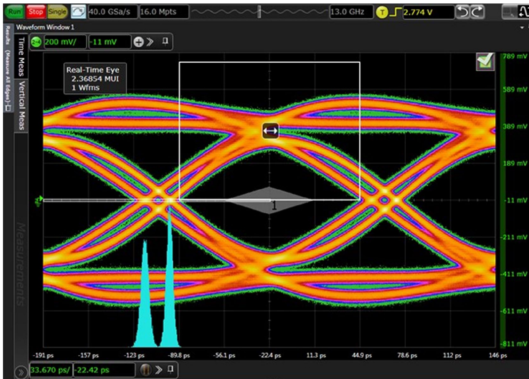
Fig. 9. HDMI 2.1 6 Gbps TMDS eye diagram, PCB with device; typical values
