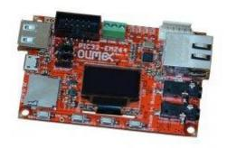
Open Source Hardware board with PIC32 processor
