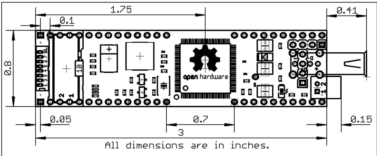
Note that the iMX233-OLinuXino-NANO board has a 6-layer PCB. The three highest elements on the board in order from the tallest to the shortest are: vertical USB HOST – 16.2mm (0.640") over the pcb; UEXT connector – 13.6mm (0.525"); U\_DEBUG pins – 12.0mm(0.464").
