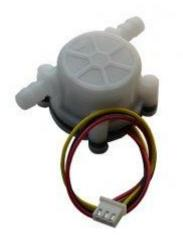
1/8" High precision water flow meter / water flow sensor with Hall effect pulse switch. Can be used in a coffee machine; a water dispenser; a water purifier flow meter; etc.
