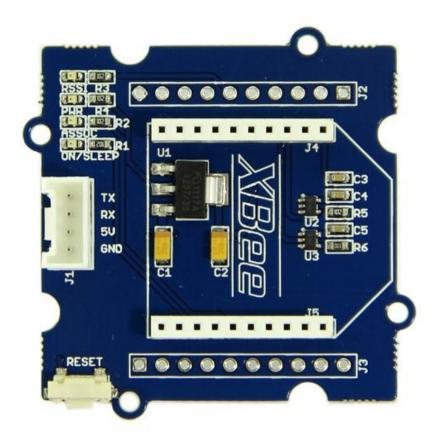
Grove - Bee Socket is an adapter of Xbee serials which can connect wireless modules with Arduino, such as WIFI Bee, RF Bee, Bluetooth Bee, etc. It is Arduino compatible and more effective to conduct operations of peer to peer and mesh network ran by wireless modules. Regulator CJT1117 guarantees Xbee of stable 3.3 voltage. LEDs can perform work modes of the grove clearly. Grove-Bee Socket has the same functions as XBee Shield. Grove-Bee Socket
