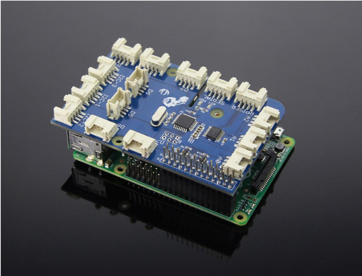
GrovePi is an add-on board that brings Grove Sensors to the Raspberry Pi. As a new version of GrovePi. It adds support for the newly RaspberryPi Model B+ and Model A+. There are three mounting holes can perfect match all version of Raspberry Pi. Camera cable outlet hole. It also improves the voltage level converting sub circuits.
