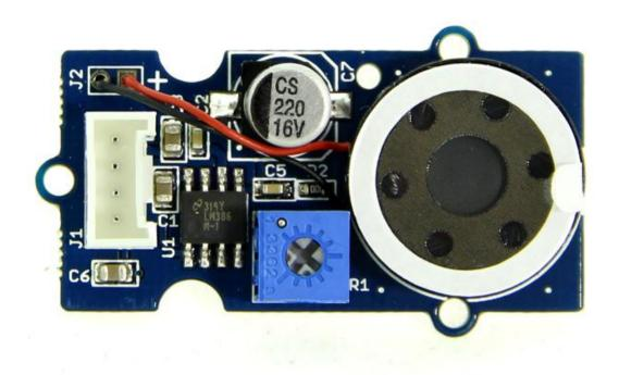
The Grove- Speaker is a module which consists of power amplification and voice outputs. The loudness can be adjusted by the on-board potentiometer. With different input frequencies, the loud-speaker generates different tones. Coding the music into arduino, DIY your own music box!
