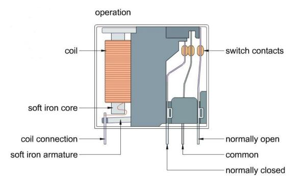
You may see that the common terminal and the normally closed terminal have continuity When the coil of the relay is at rest.
