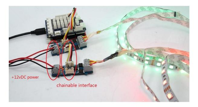
4.In cases that you want to utilize the cascade feature, prepare another driver and strip first. Then use a Grove cable to connect the Grove socket marked "out" on the first board and the Grove socket marked "IN" on the second board. Done. Two strips will shine in sync now.
