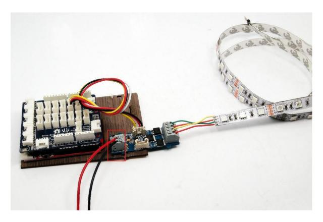
3.Connect the 12V DC or 9V DC power wires to the 2 pin terminal.
