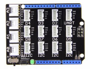
Arduino Uno is the most popular Arduino board so far, however it is sometimes frustrating when your project requires a lot of sensors or Leds and your jumper wires are in a mess. The purpose of creating the Base Shield is to help you get rid of bread board and jumper wires. With the rich grove connectors on the base board, you can add all the grove modules to the Arduino Uno conveniently! The pinout of Base Shield V2 is the same as Arduino Uno R3.
