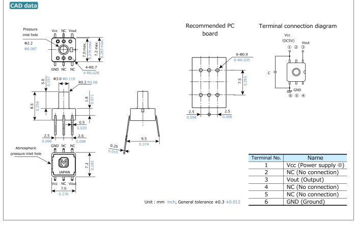
• Standard type M package (Terminal direction : SMD terminal Pressure inlet hole length : 5 mm 0.197 inch) ADP52 1
