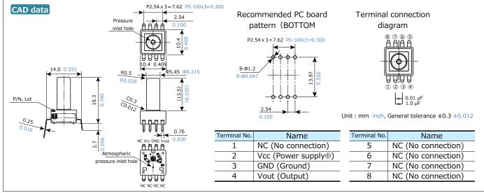
• Low pressure type P package (Terminal direction : DIP terminal, Pressure inlet hole length : 15.6 mm 0.614 inch) ADP51B63
