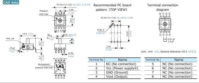
• Low pressure type L Package (Terminal direction : DIP terminal, Pressure inlet hole length : 13.5 mm 0.531 inch) ADP51B62
