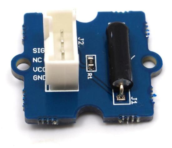
The Grove-Tilt Switch is the equivalent of a button, and is used as a digital input. Inside the tilt switch is a pair of balls that make contact with the pins when the case is upright. Tilt the case over and the balls don't touch, thus not making a connection. It is wired to the SIG line, NC is not used on this Grove.
