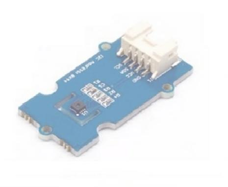
Grove - Temp&Humi Sensor(SHT31) is a highly reliable, accurate, quick response and integrated temperature & humidity sensor. The sensor(chip) used in the module is designed with Sensirion's CMOSens<sup>®</sup> technology. The chip is well calibrated, linearized and compensated for digital output.
