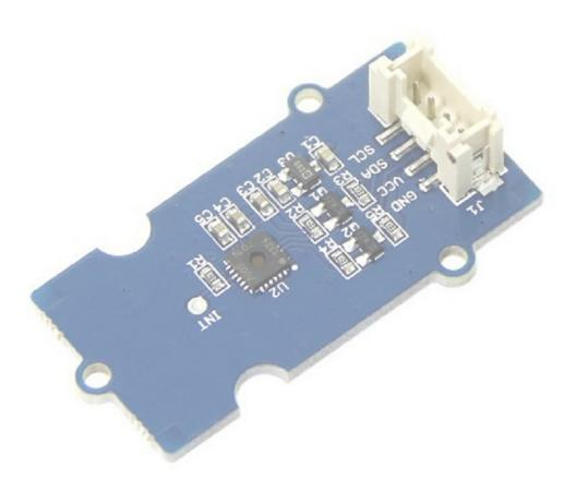
This is a multifunctional sensor that gives you temperature and relative humidity information at the same time. It utilizes a TH02 sensor that can meet measurement needs of general purposes. It provides reliable readings when environment humidity condition in between 0-80% RH, and temperature condition in between 0-70°C, covering needs in most home and daily applications that don't contain extreme conditions.
