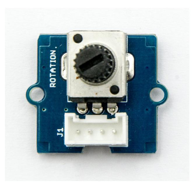
The rotary angle sensor produces analog output between 0 and Vcc (5V DC with Seeeduino) on its D1 connector. The D2 connector is not used. The angular range is 300 degrees with a linear change in value. The resistance value is 10k ohms, perfect for Arduino use. This may also be known as a "potentiometer".
