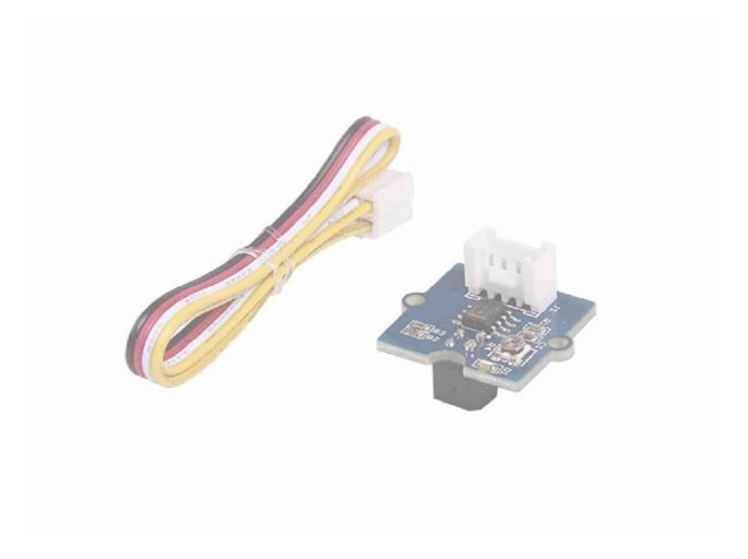
Grove - Infrared Reflective Sensor is used to detect the presence of an object within a specific range. The sensor consists of an IR LED and a photosensor (phototransistor) pair. The light emitted by the IR LED gets reflected by any object placed in front of the sensor and this reflection is detected by the photosensor(phototransistor). Any white (or lighter) colored surface reflects more than black (or darker) colored surface.
