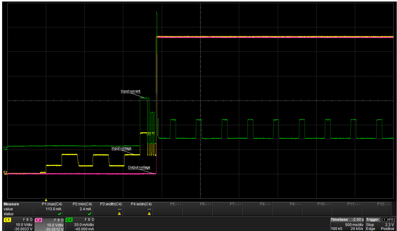
Figure 17. No Load Start-up, MPS Circuit Turned ON
