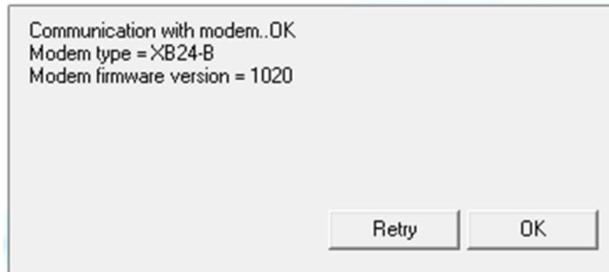
Figure 3: Testing the connection to the XBee module
