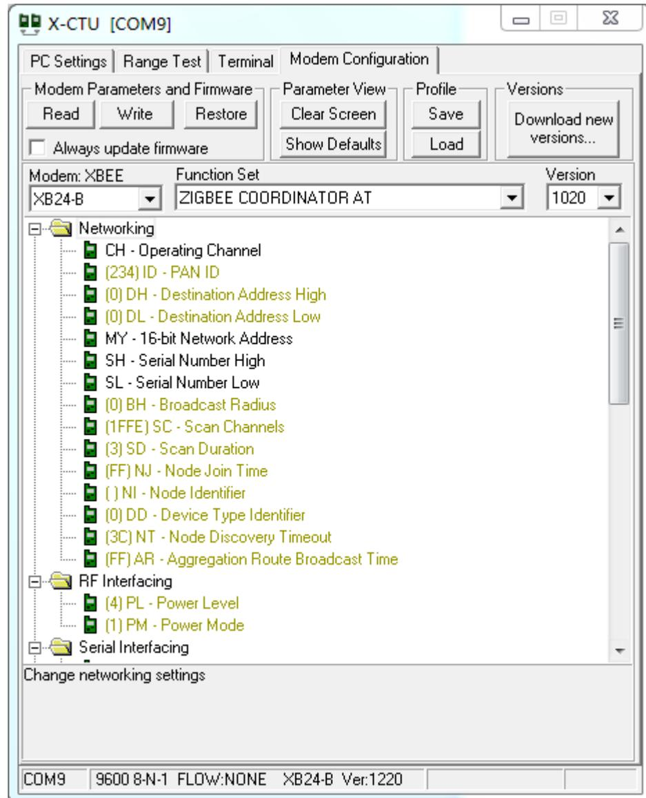
Figure 4: Getting the current parameters of XBee-A
