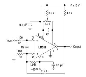
Figure 17. Conventional Technique for Adding Hysteresis
