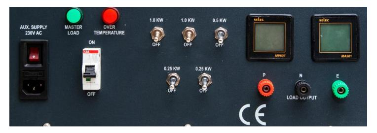
MASTER LOAD (Green Indicator): Indicates load is in ON condition and load step switches can be activated
