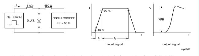
Input signal: forward pulse rise time  $t_r$  = 20 ns; forward current pulse duration  $t_p \ge 100$  ns; duty cycle  $\delta \le 0.005$
