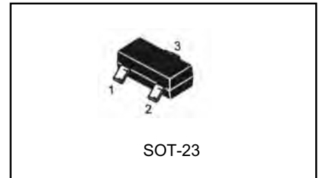
SOT-23 1: Ref; 2: Cathode; 3: Anode
