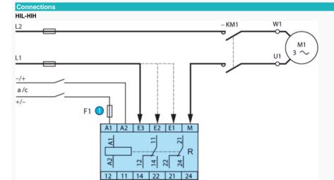
NB: When controlling DC current from the same source supplying terminals A1 and A2, terminal M must be connected directly to the "minus" pole of this power supply.
